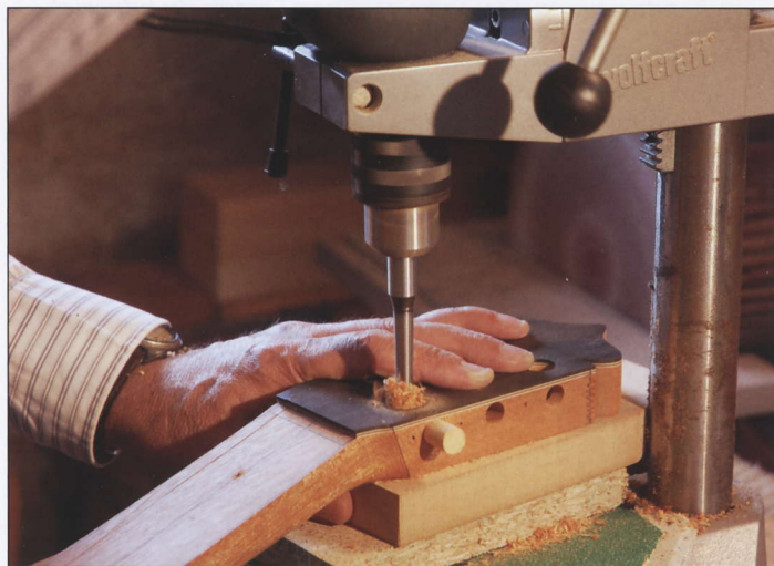
Above: Classical guitars in granadillo (at left) and rosewood. One is an endangered species, the other is not. The Der Jung tuners are elegant and a good value. Below: Dowels prevent splitting the barrel holes when drilling slot ends. Bottom: Scalloping brace ends for a classical guitar.
