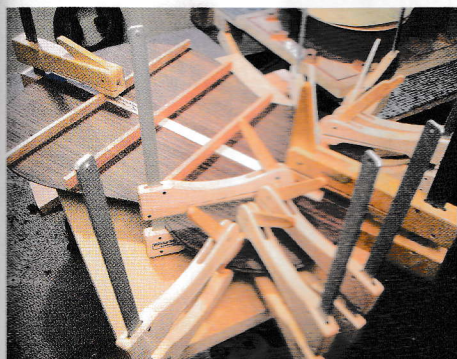
27 Clamping the back braces into place
