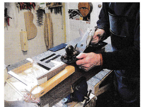
17 My old 5½ plane is used to true the back join
