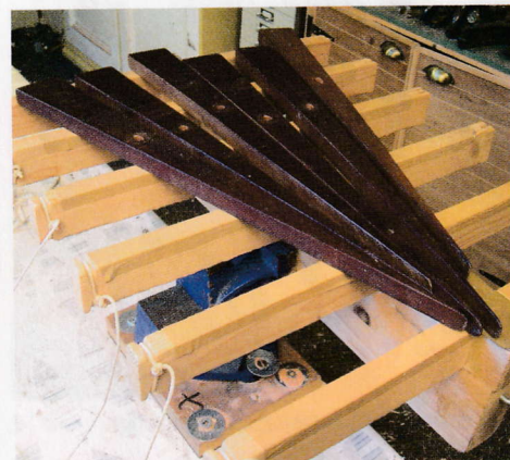
19 The wedge and lace jig for joining backs and soundboards
