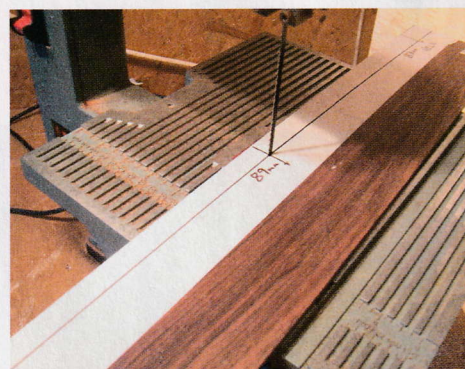
8 The correct taper is cut into ribs
