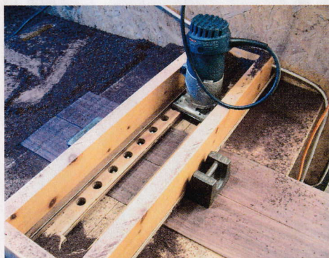
6 A homemade rib thicknessing jig
