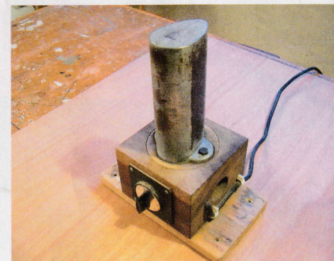
9 A commercially available bending iron
