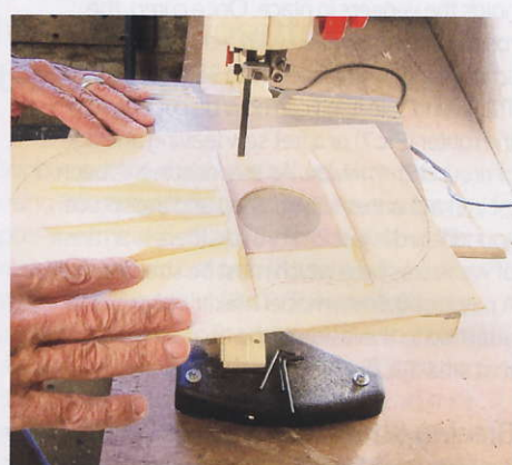
STEP 14. Cutting the front to shape
