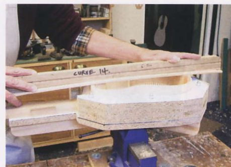
STEP 29. Sanding the 3mm lift
