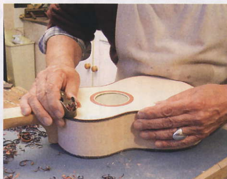
STEP 41. Trimming the bindings flush
