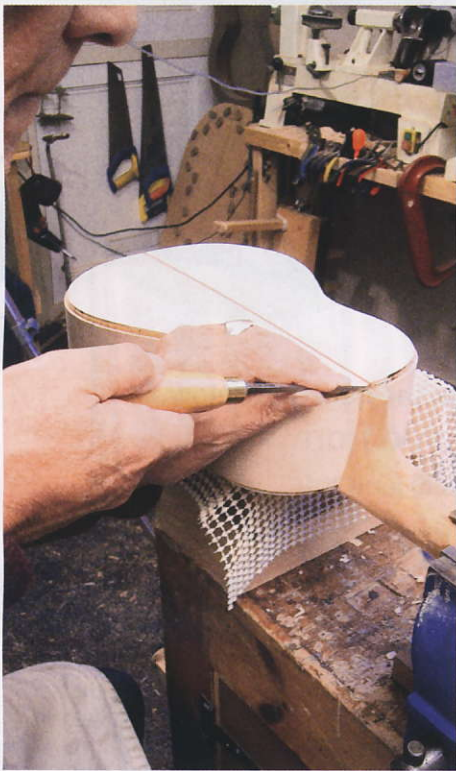
STEP 38. Chiselling the slots
