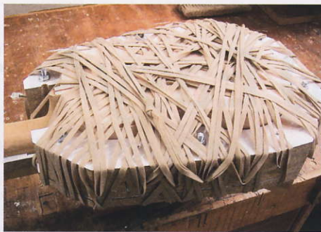
STEP 36. Elastic bands hold the back in place
