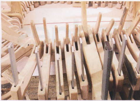
STEP 35. Clamping the back in place
