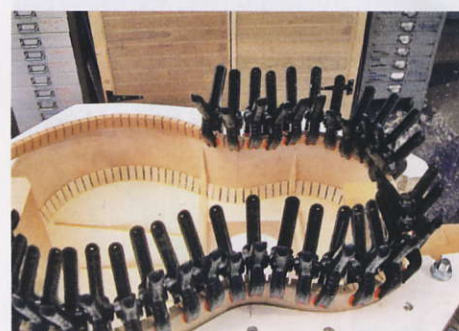
STEP 32. Clamping the kerfed lining into place
