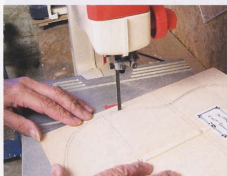
STEP 33. Cutting the back to shape
