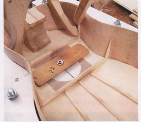
STEP 20. Clamping the long tentellones
