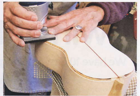
STEP 37. Cutting the binding and purfling channels
