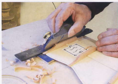
STEP 27. Gabling the back braces
