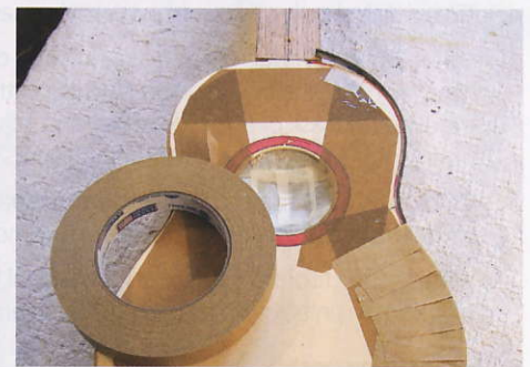
STEP 40. The bindings and purflings held in place with masking tape
