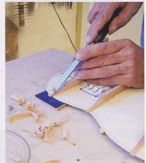
STEP 26. Scalloping the back braces
