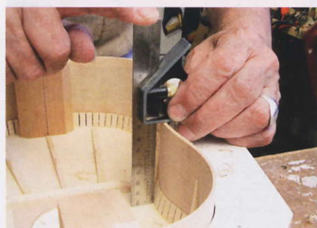
STEP 31. Ensuring opposite sides are equal height
