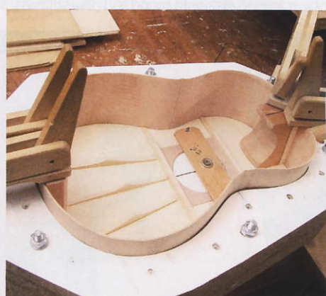
STEP 17. Fitting the front of the ukulele
