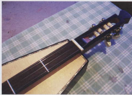
STEP 53. The top nut is made from bone
