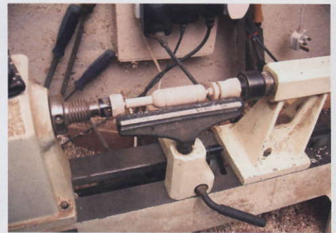
STEP 54. Turning a noter on the lathe
