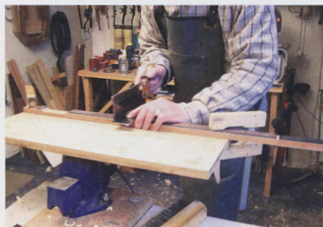
STEP 33. A dovetail saw cuts fret slots well
