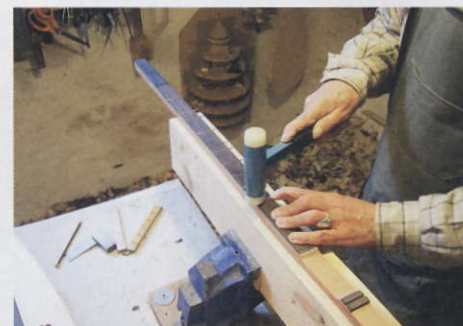
STEP 35. A dead blow hammer is good for fretting
