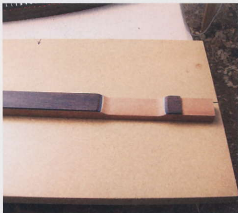
STEP 30. The scoop cut into the lower end of the neck
