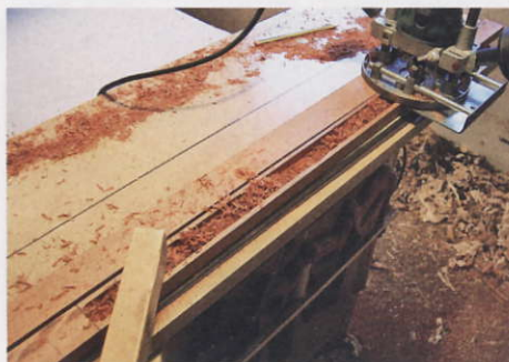
STEP 28. The neck is then hollowed out below the fingerboard
