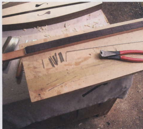
STEP 31. Frets being cut from straight lengths of wire
