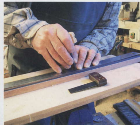
STEP 32. A pinprick made with a scribe is a guide to the exact fret position
