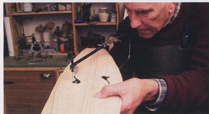
STEP 15. The soundholes are cut out with a long reach fretsaw
