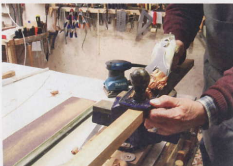
STEP 27. The neck is planed to dimension from a billet of mahogany
