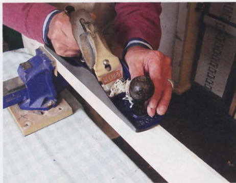
STEP 11. The inside edges of the soundboard are planed square...
