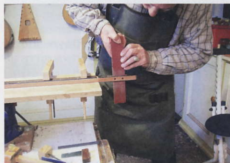
STEP 42. The insides of the string slots are cleaned up
