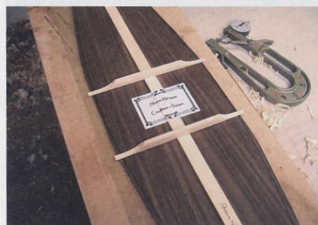
STEP 45. The inside of the back is strengthened with cross-banding and struts
