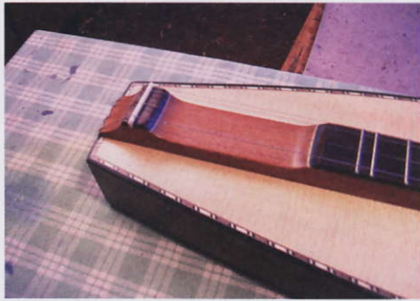
STEP 52. The bone saddle is located at the tail end of the neck
