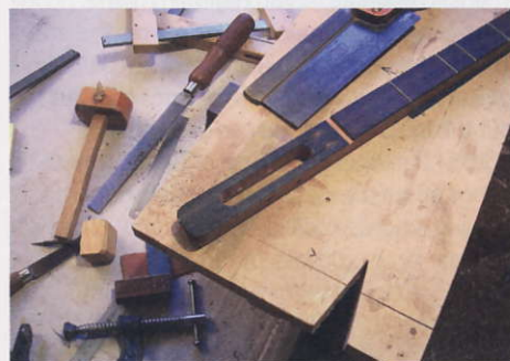
STEP 41. Two small saw cuts guide the chisel for the 'ski slope'
