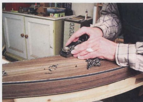
STEP 48. The bindings are trimmed roughly flush with the ribs...
