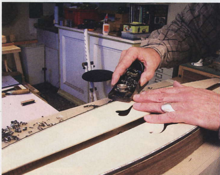
STEP 22. The edges of the bindings are brought flush with a small plane
