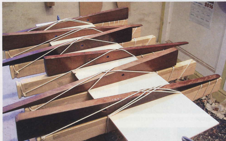
STEP 13. The soundboard halves in the wedge and lace jig
