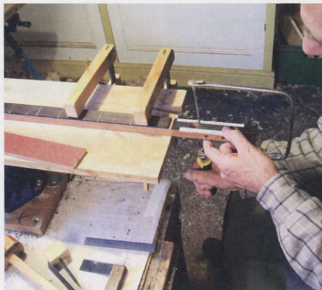
STEP 40. The slots are cut out with a coping saw
