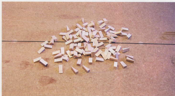
STEP 17. Tentellones to hold the soundboard in place
