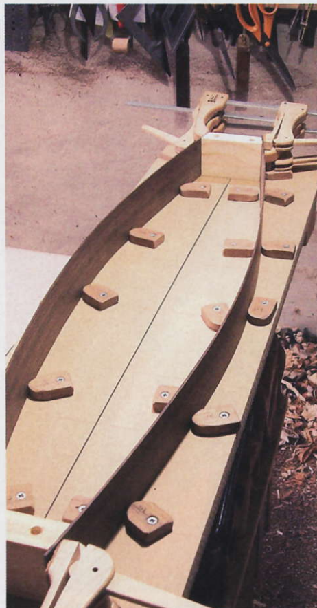
STEP 9. The ribs are attached to the end blocks
