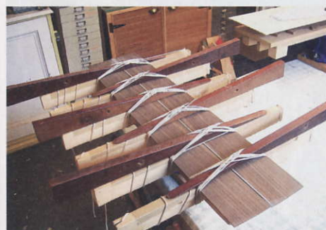
STEP 44. The two halves of the back and centre strip in the wedge and lace jig
