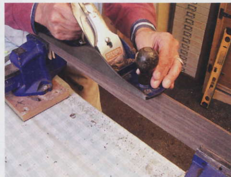
STEP 6. Planing the edges of the ribs...
