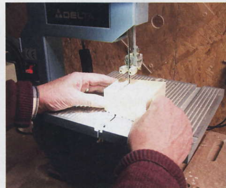
STEP 8. Cutting end blocks on the bandsaw
