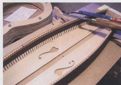
STEP 46. Small housings are cut into the linings to receive the ends of the struts
