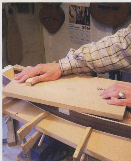
STEP 26. ... and are then sanded exactly flat
