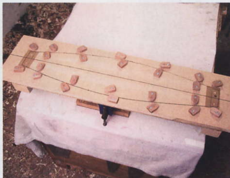
STEP 5. Cams are used to hold the instrument's shape
