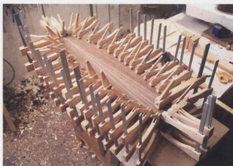
STEP 47. The back held in place with cam clamps
