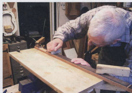
STEP 34. Testing the depth of the slot
