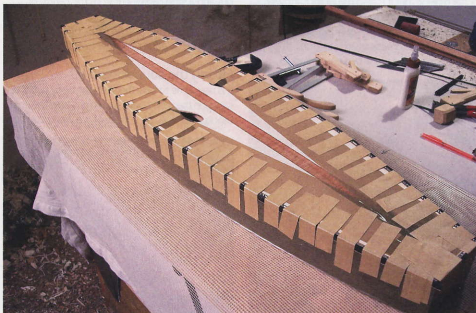
STEP 21. Bindings and purflings are held in place using masking tape
