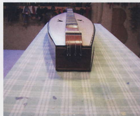
STEP 51. The hitch pins in the tail
