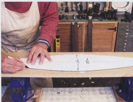
STEP 4. Marking the outline onto the face of the workboard
