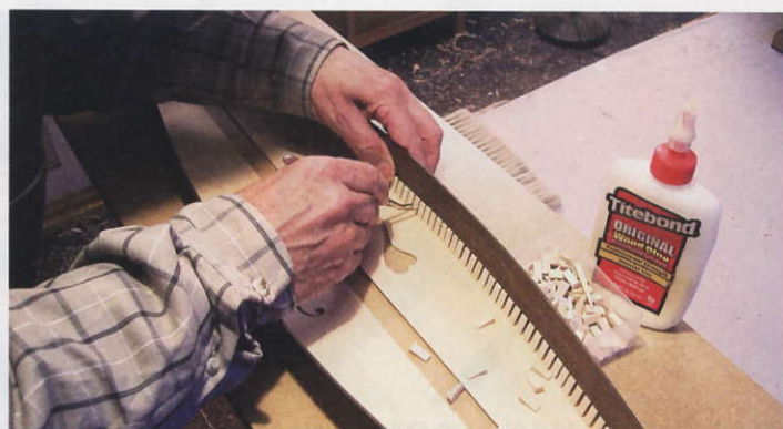
STEP 18. Tweezers are used to put the tentellones into position
