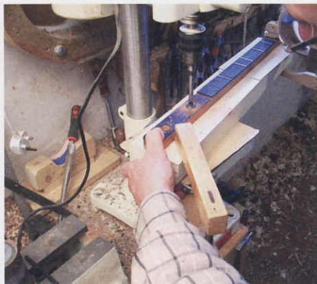
STEP 39. The string slots start with a hole at either end of the headstock
