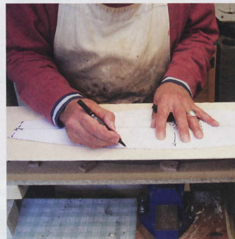
STEP 14. The outline of the dulcimer is transferred onto the soundboard
