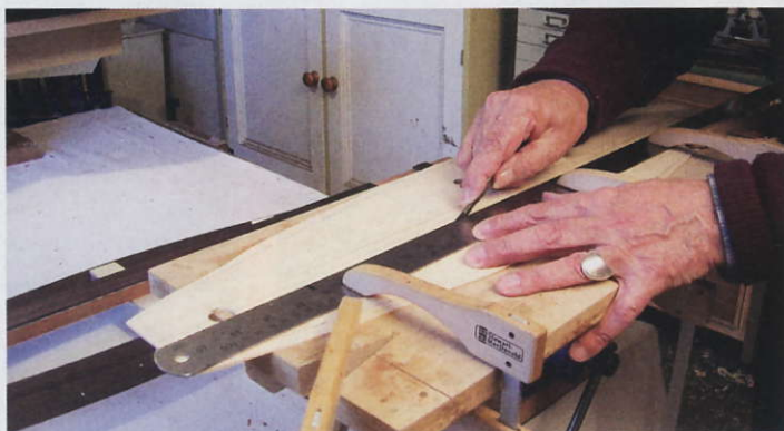
STEP 16. To aid resonance a strip of spruce is removed from the centre of the soundboard
