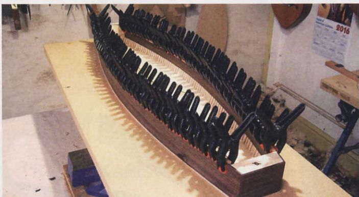
STEP 24. Kerfed linings held in place with mini clamps
