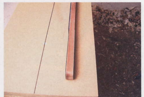
STEP 29. The headstock has ebony veneers facing the front and back
