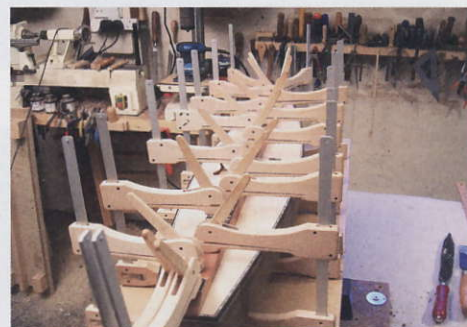
STEP 43. The neck and fingerboard are then clamped into place
