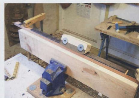
STEP 38. They need to have their ends angled to around 30°
