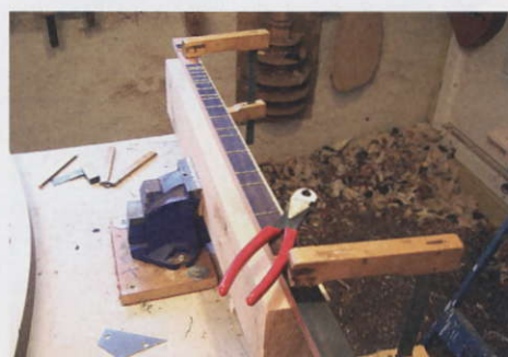
STEP 36. The fret ends are trimmed so they are roughly flush...
