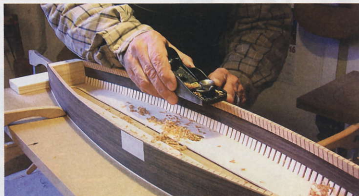
STEP 25. The edges of the linings are trimmed to the edge of the ribs...
