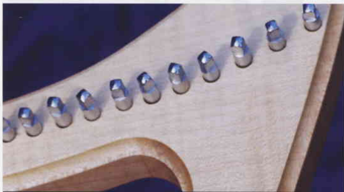
The tuning pins and tuning lever. Each pin has a 1:40 taper and is made from nickel silver.
