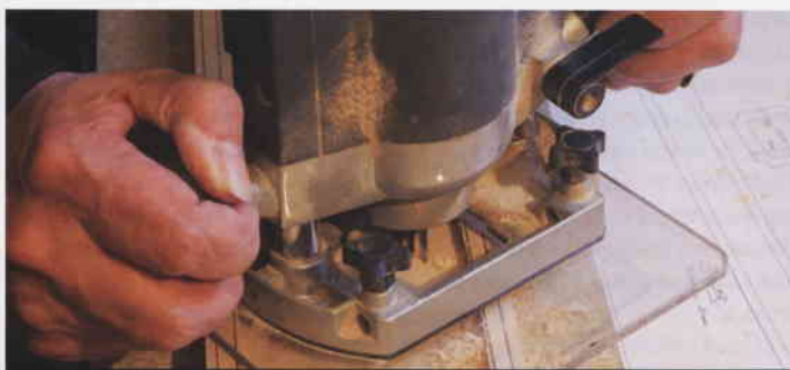
Routing out the hollow in the soundbox with a home-made Perspex base to allow a clear view of the process.
