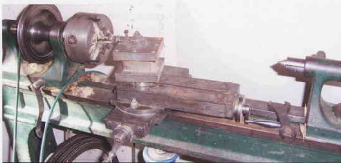
The 19th-century 'gentleman's lathe' used to turn the bridge pins. The lathe is driven by leg power!
