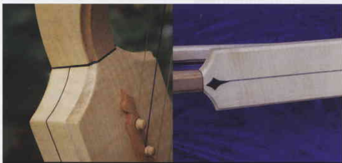
Between each half of the soundbox is a leaf of black maple veneer which gives a clean inlay line when the two halves are joined. Also, the inlay work on the back of the harp.
