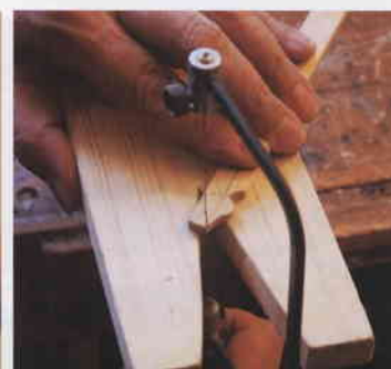
Shaping the ends of the string bar.
