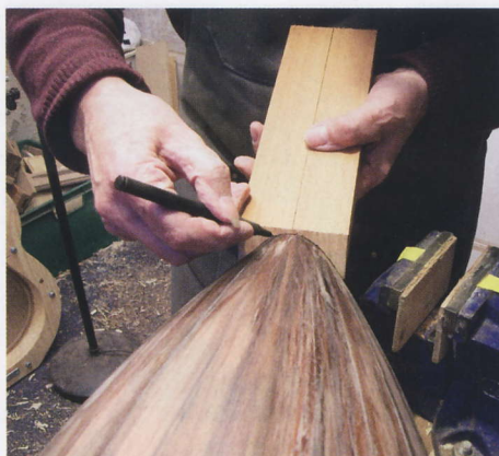
19 The outer curve of the neck is scribed following the line of the bowl
