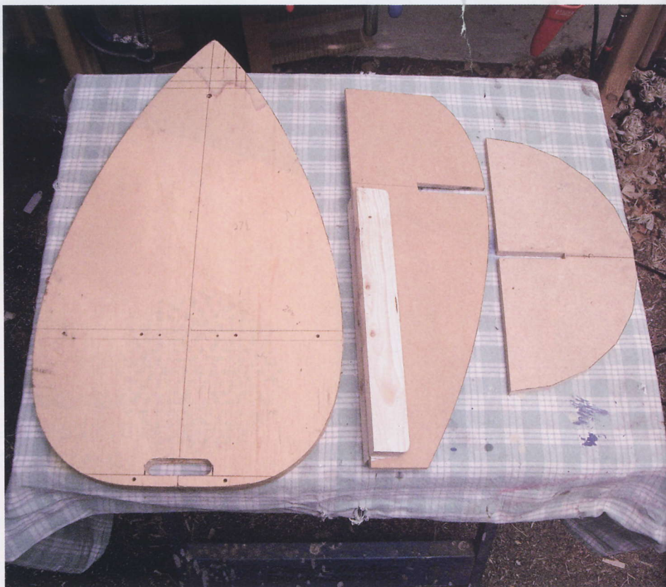
2 The components of the bowl former
