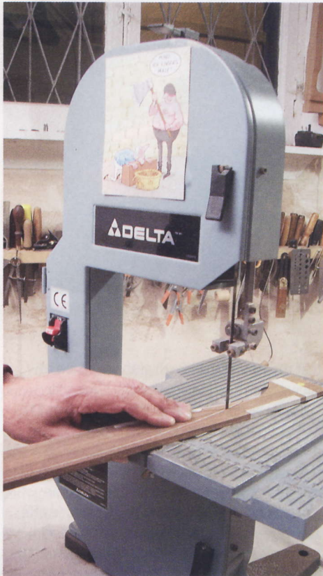
9 Cutting the ribs out on the bandsaw, two at a time
