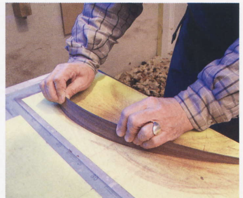
11 A slight angle is cut into the edges of each rib
