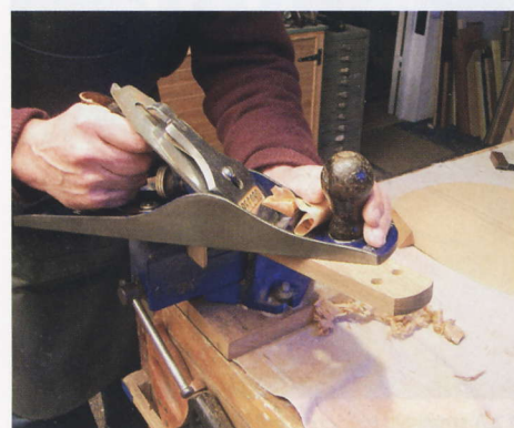
22 Tapering the peghead with a No.5 1/2 plane
