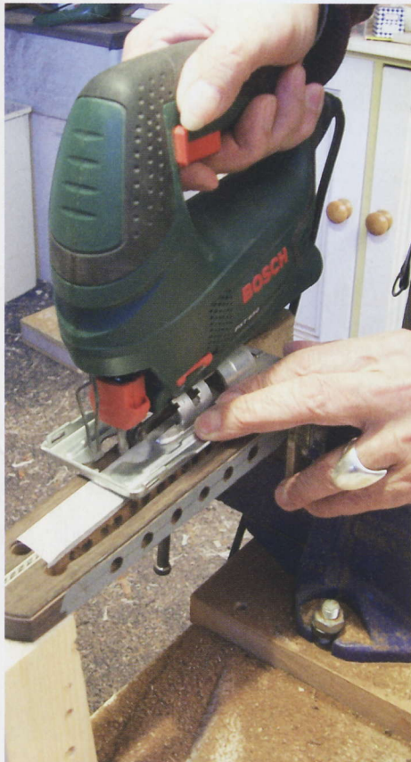
27 A jigsaw cuts out the string slots with ease
