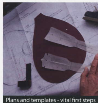
Plans and templates - vital first steps
