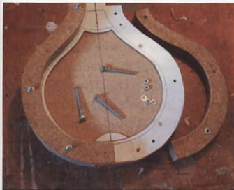
The mould constructed from chipboard and held together with coach bolts
