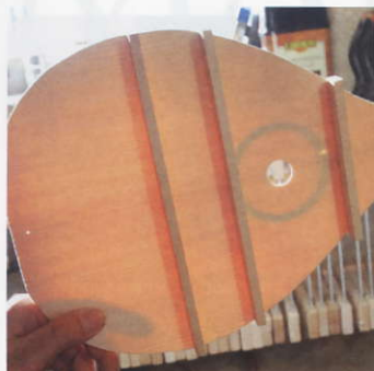
Masking tape pulled tight holds the bindings firmly in place
