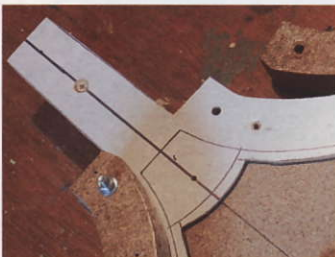
The centre line on the mould must match up exactly with the centre of the neck
